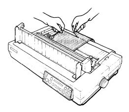
Press the ON LINE button to set the printer off line. Then press the FORM FEED button to eject the labels. (Remember not to use the LOAD/EJECT button to eject labels.)
